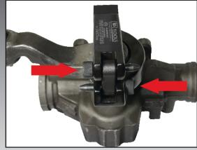
Tip: On the 1988-2000 4X4 applications it is best to insert the pins in the direction shown.
