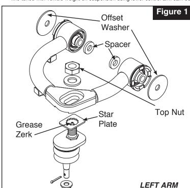
NOTE: Camber and caster can be set with the SPC upper control arm, as well as the lower control arm cam bolts. In most cases, it is recommended that the lower cam bolts be set to their neutral position. This way they can be used to fine-tune caster.
